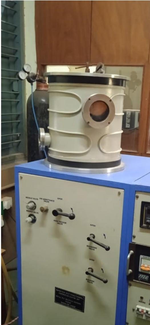
The **Magnetron Sputtering/Thermal Evaporation coating unit** is a sophisticated piece of equipment used for depositing thin films and coatings on substrates. This unit integrates two primary deposition techniques: magnetron sputtering and thermal evaporation, each offering unique advantages for various applications in materials science, electronics, optics, and engineering.
